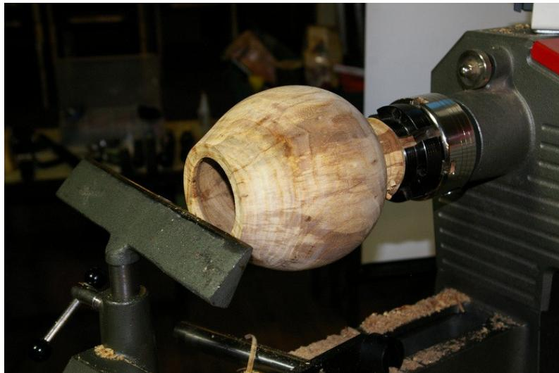
The base of the vessel is left thick at this stage to provide additional support during the hollowing phase. Initial roughing out of the interior is followed by working down in 2" (50mm) steps taking the thickness down to just over  $\frac{1}{8}$  inch (4mm). Remember that all this work is being done in an end grain piece. Tracy switched to a tear drop scraper for the final finishing of the interior.
