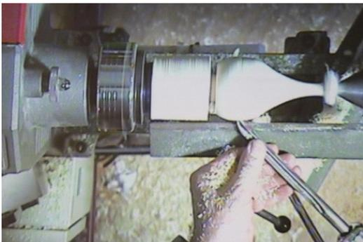
The cylinder was then mounted into a four jaw chuck retaining the tailstock support. The proportions required for the head and trunk were pencilled in and the shape of head leading into the trunk and the trunk itself were turned.
