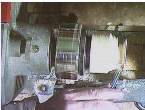
A small spigot was left in the centre which was turned to match the diameter of the hole that had been drilled in the head to receive it before it was sawn off.
