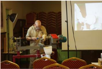
Firstly, Steve turned and finished the base of the candlestick, then onto turning the first part of the candlestick. Each operation making sure that the fitted the easily together which allowed room for the glue.
