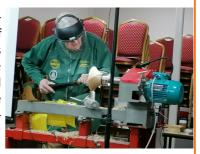
The final stage was the remounting of the bowl in Cole Jaws to turn away the recess as all turners like to have a "smooth bottom"
