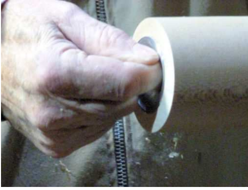
The pre-bored hole was then shaped to fit the cup that Gerry had spun previously.
