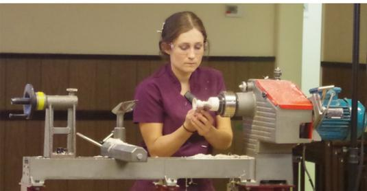
Now to turn the top of the ornament. Emma put a Jacob's chuck in the tail-stock and used a 3mm drill bit to make a pilot hole, then enlarged it to 4mm. This was to take the wire, which has tiny LED lights incorporated at intervals. These often have bits sticking out which may mean the hole has to be made bigger. It is important that the
