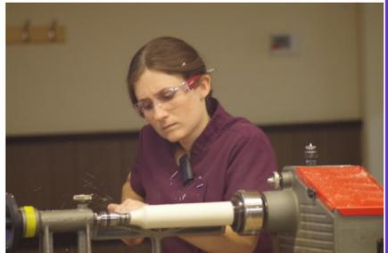
Emma has adapted her turning technique to overcome the limitations of her height, not only raising her elbows and even standing on tiptoe, but grinding her tools to facilitate access to the wood. For example, she uses a large spindle roughing gouge which has a bevel close to 90°.
